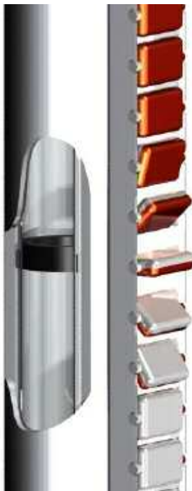
Cut-Away Section of Float Chamber
